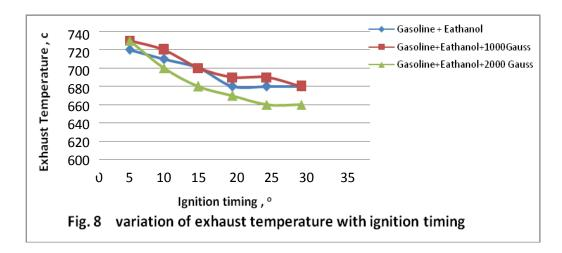
With the presence of magnetic field, the internal energy of the fuel increases which means that molecules fly apart easier, join with oxygen easier and burn more completely. The magnetic field can change the spin state of hydrogen molecules in the fuel (converted from para-hydrogen to ortho-hydrogen) which greatly enhances the energy of the atom and increases fuel reactivity leading to higher engine output, better fuel economy and lower amount of hydrocarbons and carbon monoxide in the exhaust.
